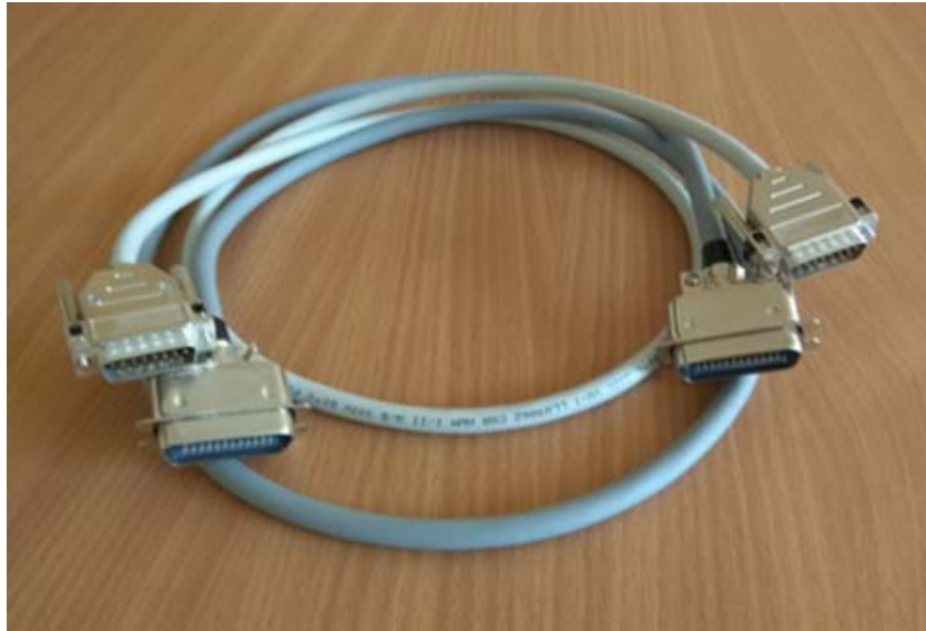
Fig. 1.35. Cables for connecting hardware modules
