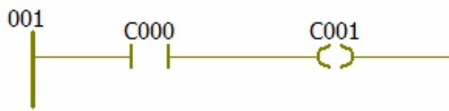
Fig. 4.45. Basic components of Ladder Diagram
