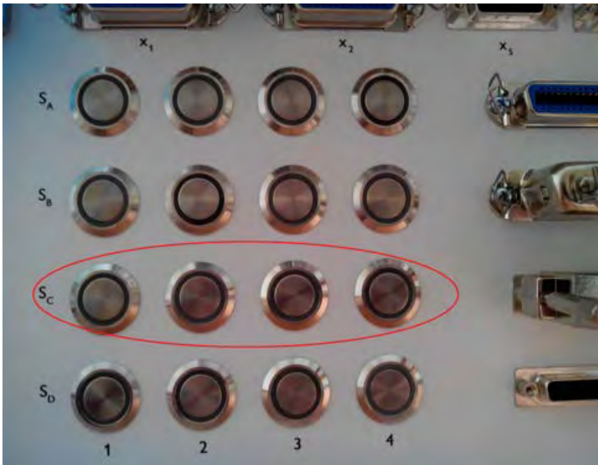
Fig. 4.32. Block of LEDs of output global variables in the third hardware module
