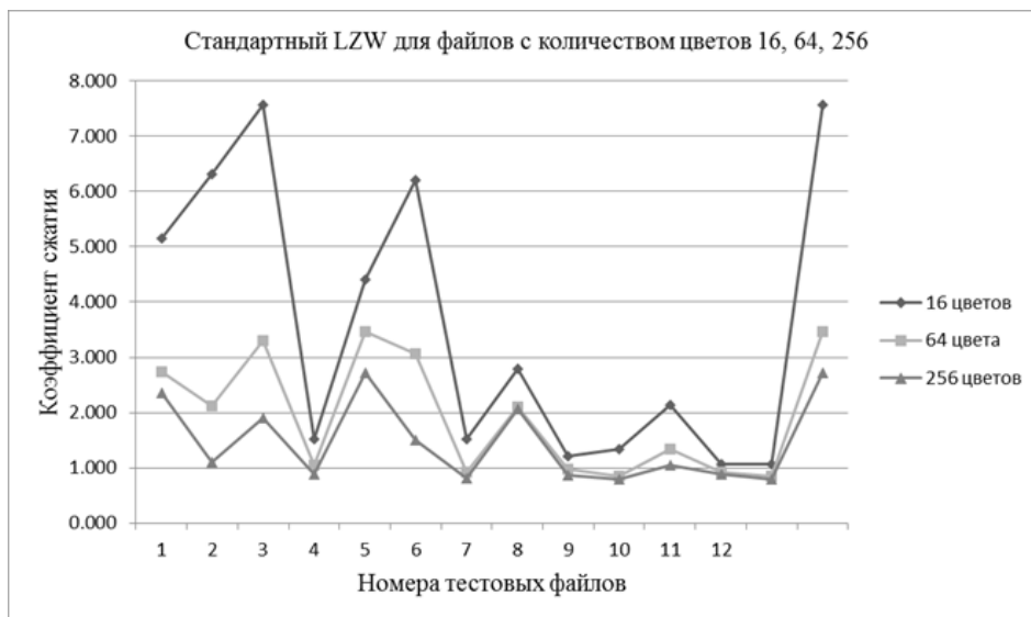
Fig. 5. LZW compression ratio diagram
