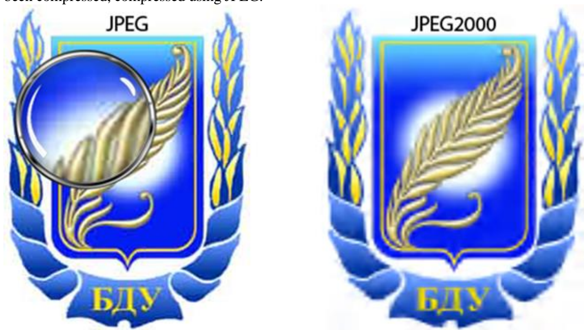
Fig. 4. Comparison of images compressed with JPEG and JPEG-2000
