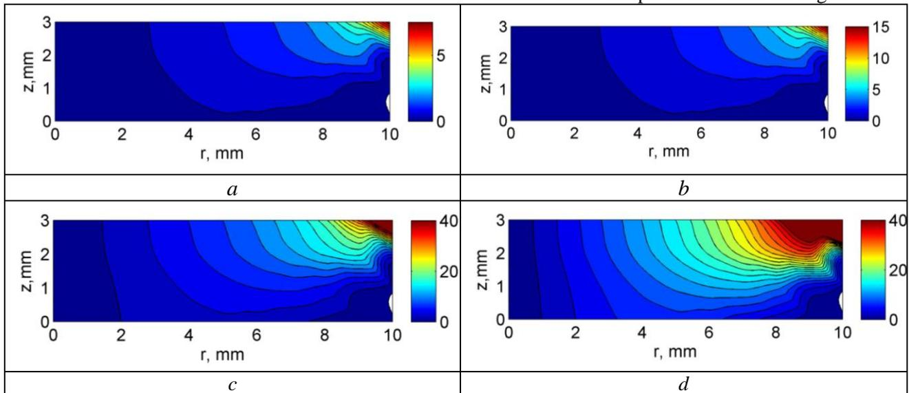
Fig.2 The von Mises strain distribution in the axial cross-section of the sample for the compression pressure  $p = 1.1GPa$  and for the rotation angle equals to: a-  $\frac{\pi}{4}$ , b-  $\frac{\pi}{2}$ , c-  $2\pi$ , and d-  $4\pi$ .
