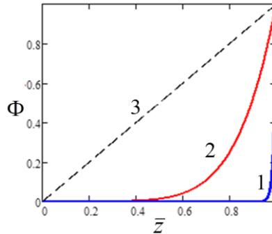
Fig.5 The dependence  $\Phi(\bar{z}) = \bar{z}^k$  for different values of the index  $k$ : 1-  $k = 100$ , 2-  $k = 5.2$ , 3-  $k = 1$  (coincide with the velocity field usually used for HPT, uniform strain distribution on the axial direction).
