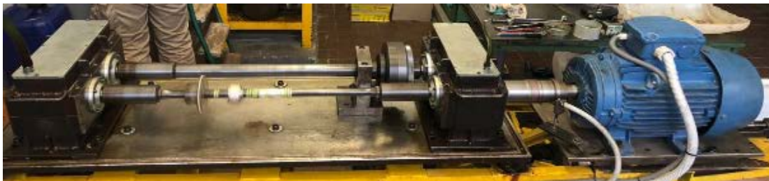
Fig. 1. Measuring device Tribotestor M'06 and a detailed view of the measuring head and test samples
