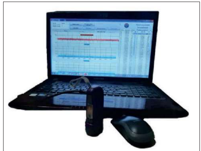
Fig. 1. A sample of the «Trembita-Corona» acoustic monitoring device
