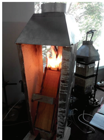
Fig. 5. Device for determining the index of flame spread over the wood surface
