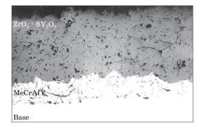
Fig. 8. The microstructure of barrier coating. Reproduced with permission from M. Hetmanczyk et al., J. of Ach. Mater. Manuf. Engin., 24, No.1: 372 (2007); https://www.researchgate.net/ publication/40804836\_Advanced\_ materials\_and\_protective\_coatings\_in\_aero-engines\_application. Copyright 2007, International OC-SCO World Press [101]
