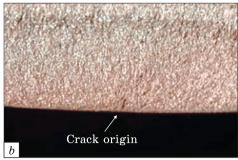
Fig. 4. (a) Fatigue cracks, (b) crack initiation, (c) fatigue striations in the crack propagation zone. Reproduced with permission from M. Sujata and S.K. Bhaumik, J. of Fail. Anal. Prev., 15: 45 (2015). Copyright 2015, Springer [43]
