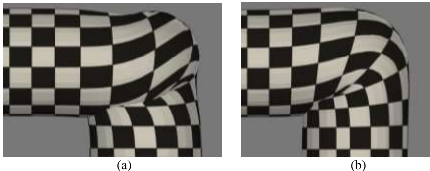
Fig. 6. Left is an artifact, that arises, when bending and twisting same the joint simultaneously.
