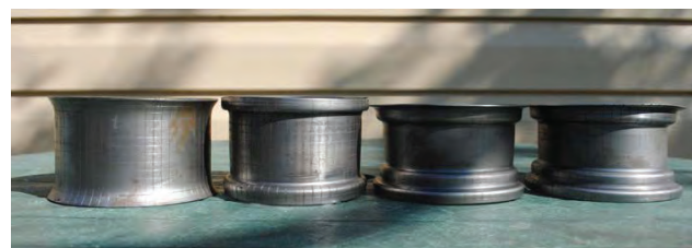
Fig. 6. Profiles of the models of the rims of wheels in the transitions of radial-rotary profiling for the standard size 5.5Fx20
