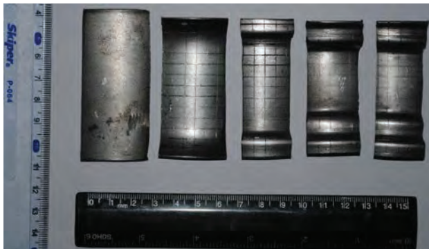
Fig. 7. Templates in the transitions of profiling for the model of the wheel rim 5.5Fx20
