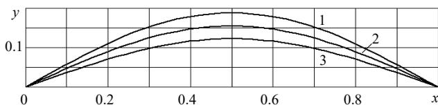
Fig. 2. Railroad track curvilinear sections: 1 –  $\varphi_0=30^\circ$ ; 2 –  $\varphi_0=25^\circ$ ; 3 –  $\varphi_0=20^\circ$
