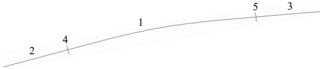
Fig. 1. The proposed structure of the curvilinear section of a railroad track: 1 – curvilinear section; 2, 3 – rectilinear rails; 4, 5 – boundary points
