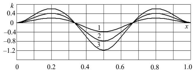
Fig. 5. Outer rails' elevation curvature distribution curves: 1 –  $\varphi_0=30^\circ$ ; 2 –  $\varphi_0=25^\circ$ ; 3 –  $\varphi_0=20^\circ$
