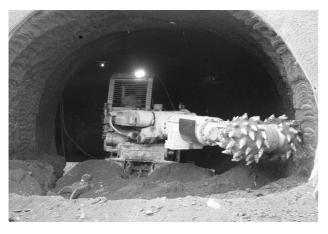
Fig. 3. A roadheader during work procedure
