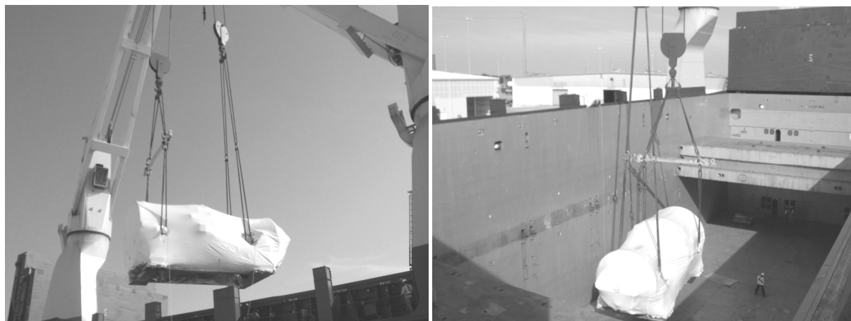
Picture 5 — Turbine loading/discharging operation
