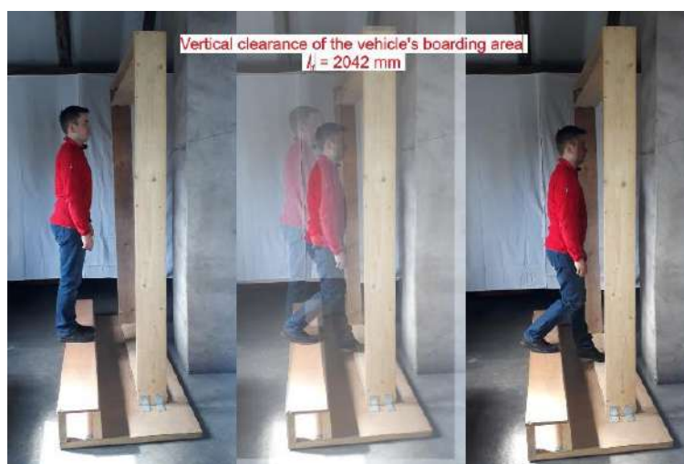
Fig. 17 – Vehicle boarding simulation with vertical clearance h_1 = 2042 mm
