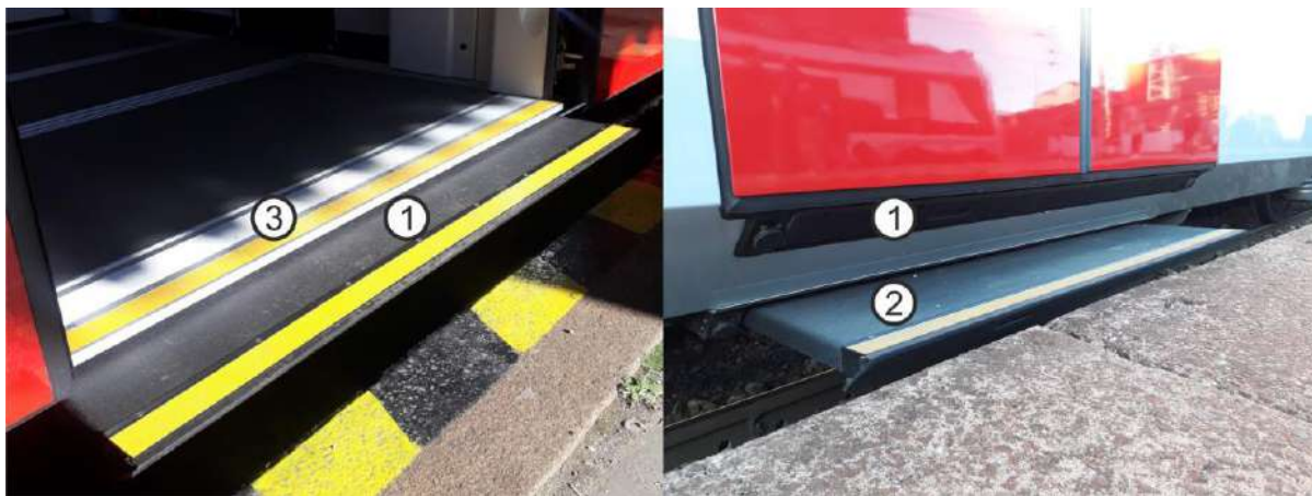
Fig. 3 – Extendable steps on the vehicle 14Ev from Škoda Transportation
