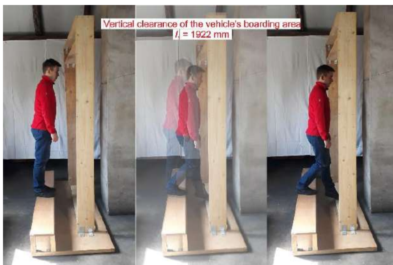
Fig. 16 – Vehicle boarding simulation with vertical clearance l_1 = 1922 mm
