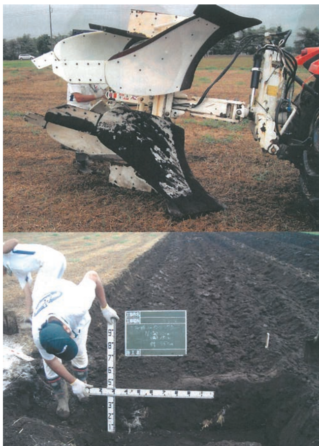
Fig. 1. Deep-plowing method with soil horizons mixing (Japan)
