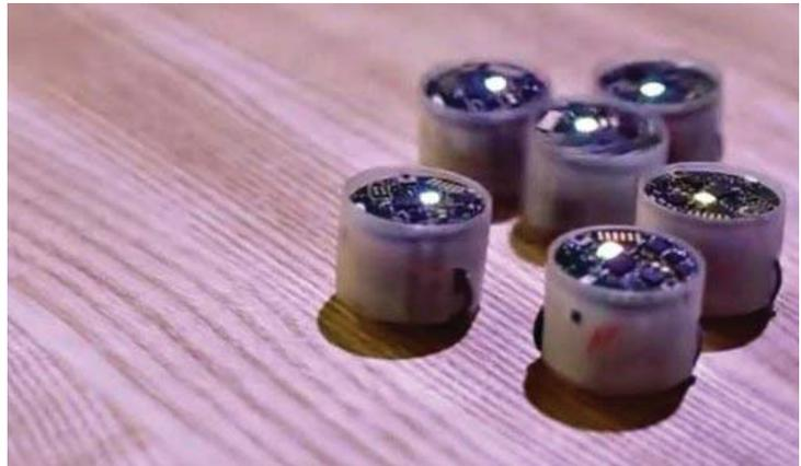
rechargeable battery, the touch sensor, a gyroscope, the optical sensor and the microcontroller. Capabilities of these microrobots are very far from capabilities of big ATLAS robots of the Boston Dynamics company, nevertheless, having united in group, they can carry out rather complex challenges.
