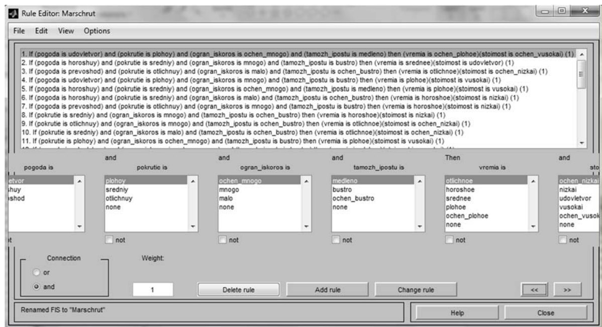
Figure 2 – The editor of the rules of the expert system of fuzzy knowledge base for selecting optimal transportation routes within the CSC framework.
