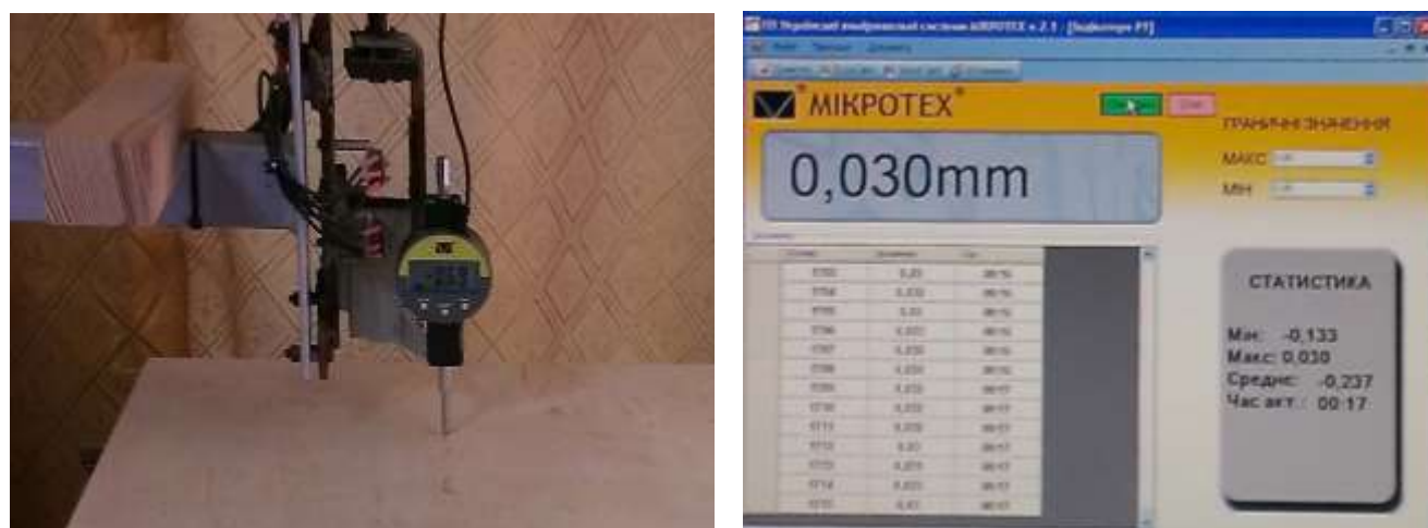
Fig. 5. CNC experimental set-up for determining shape stability of PCW-made blockboards
