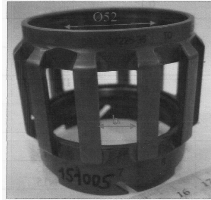
Fig. 1. Appearance of process separator with Avinit C32 coating
