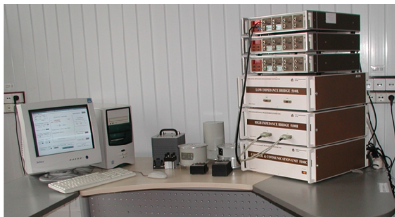
Figure 1. General view of National Standard of the units of capacitance and loss factor
