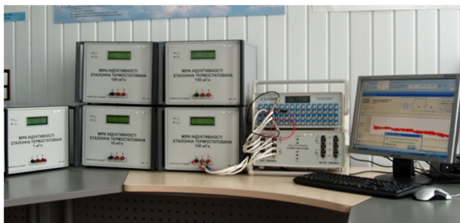
Figure 1. General view of National Standard of the units of inductance and tangent of loss
