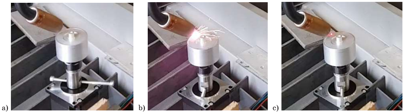
Fig. 2. The process of laser welding of the simulator sample: a) before the start; b) in process; c) stop after welding
