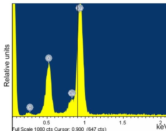
**Fig. 4** – Energy Dispersive X-Ray spectrum of deposited structure surface area
