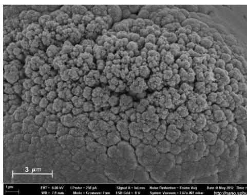
**Fig. 2** – Scanning electron microscopy image of the structure deposited out of solution composition: 0.02 M chloride copper(II), 0.5 M ammonia, 0.075 M ethylene glycol, 0.3 M potassium bromate, laser power 1300 mW, the scanning rate 0.01 mm/s, the substrate Polycore VK-96
