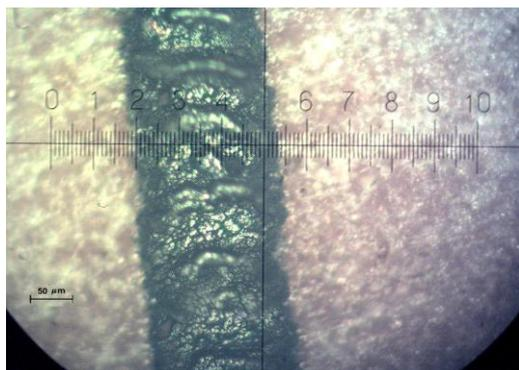
**Fig. 1** – Optical micrograph of the structure deposited out of solution composition: 0.02 M chloride copper(II), 0.5 M ammonia, 0.075 M ethylene glycol, 0.3 M potassium bromate, the power of 1300 mW, the rate of 0.01 mm/s, the substrate Polycore VK-96
