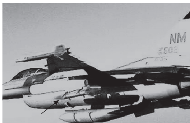
Fig. 2. Photo of an F-16 aircraft bearing one of the prototypes of ALE-50 towed decoy [7]
