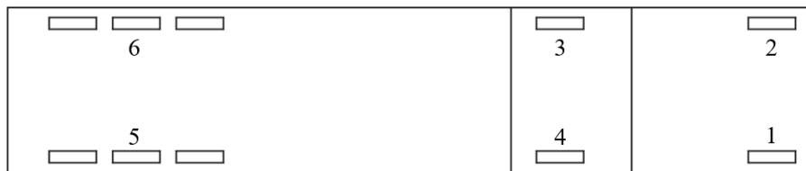
Figure 9. Numbering of the articulated vehicle wheels
