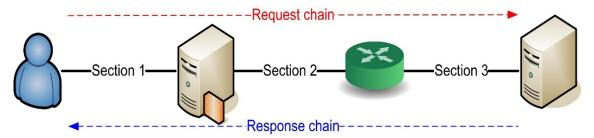
Fig. 2 An example of HTTP communication with a proxy and a gateway
