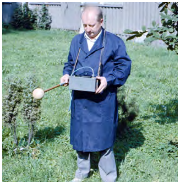
Fig. 4. EMF measurements using an universal EMF meter.
