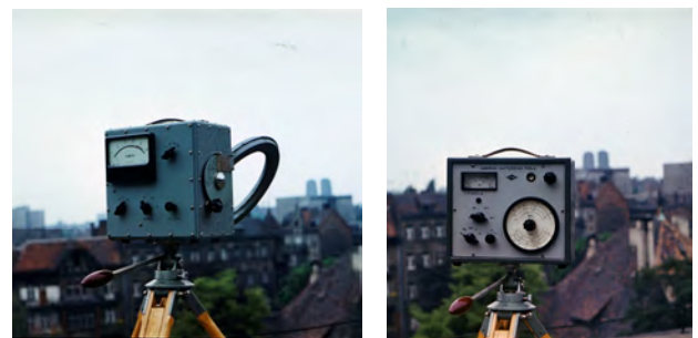
Fig. 2. A selective H-field meter (left) and E-field meter (right).
