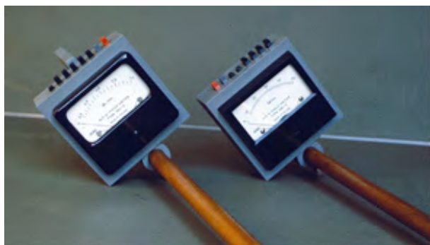
Fig. 3. An integrated wideband E-field meter (left) and H-field meter (right).
