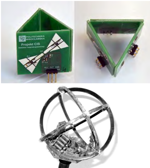
Fig. 5. Spherical E-field (above) and H-field probe (below).
