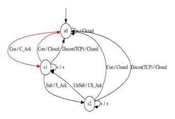
Fig. 6 – FSM model of the Mosquitto MQTT broker.
