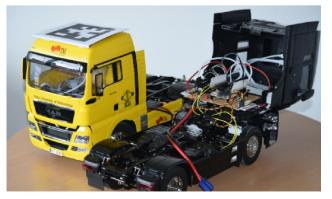
Fig. 12 – The model trucks are equipped with a BeagleBone Black board to test different scenarios on the testbed.
