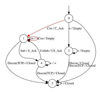
Fig. 8 – FSM model of the HBMQTT broker.
