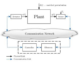
Fig. 9 – Structure of a Networked Control System.
