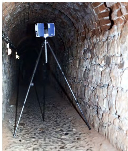
Fig. 7. Faro focus3D x 330 in the underground sidewalk
