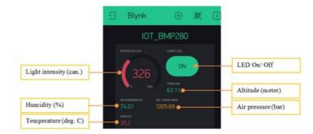
*Figure 4. The dashboard in the smartphone using Blynk app for parameter monitoring*
