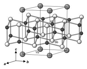
**Fig. 1** Structure of  $YbM_2Sb_2$  (M = Zn, Cd). The large lightly shaded circles are Yb atoms, the small solid circles are M atoms, and the medium open circles are Sb atoms.
