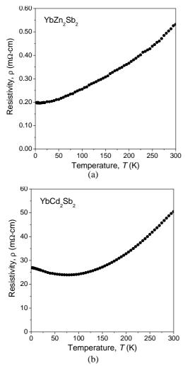
**Fig. 2** Electrical resistivity of single crystals of (a)  $YbZn_2Sb_2$  and (b)  $YbCd_2Sb_2$  measured within the *ab* plane.
