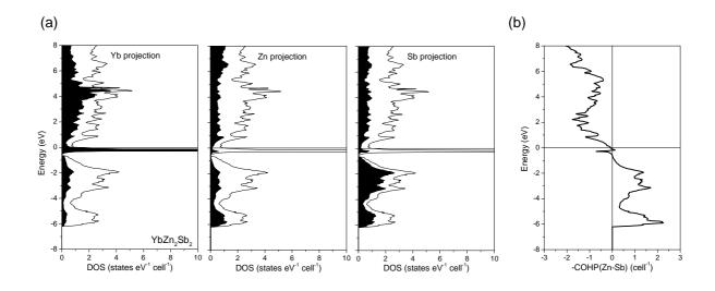
**Fig. 4** (a) Total density of states (DOS) for  $YbZn_2Sb_2$  and its Yb, Zn, and Sb projections. The Fermi level is marked by a horizontal line at 0 eV. (b) Crystal orbital Hamilton population (COHP) curve for Zn–Sb contacts in  $YbZn_2Sb_2$ .
