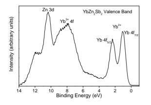
Fig. 5 Valence band spectrum of YbZn<sub>2</sub>Sb<sub>2</sub>.
