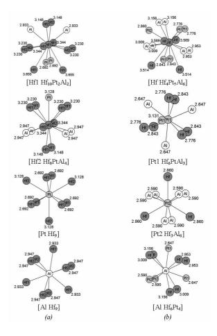
Fig. 3 Nearest-neighbor environments in the structures of  $Hf_6PtAl_2$  (a) and HfPtAl (b). Coordination polyhedra of the central atoms are indicated. Interatomic distances are shown in Å.
