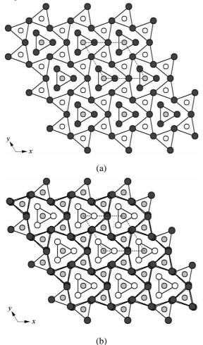
**Fig. 2** Projections of the structures of  $Hf_6PtAl_2$  (a) and HfPtAl (b) on the *xy* plane. Black circles indicate Hf atoms, grey filled circles are Pt atoms, and Al atoms are represented by white circles. The unit cells are shown using dotted lines.
