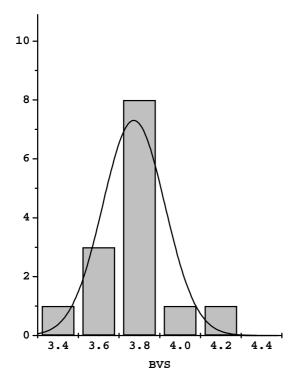
**Fig. 3** Distribution of the BVS values calculated for the Te<sup>4+</sup> ions of [TeI<sub>*n*</sub>] coordination shells using the Brese-O'Keeffe BV parameters  $r_0 = 2.76$  Å and b = 0.37 Å [21].
