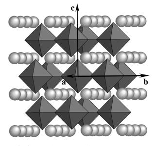
**Fig. 2** Crystal structure of K<sub>2</sub>PtCl<sub>6</sub>: [PtCl<sub>6</sub>] coordination octahedra and K atoms.
