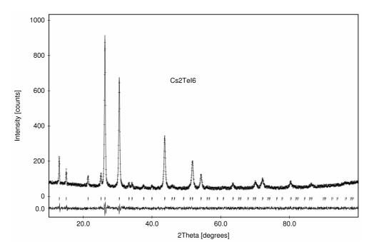
**Fig. 1** Experimental (crosses), theoretical (solid line), and difference (solid line at the bottom) powder XRD patterns for  $Cs_2TeI_6$ ; reflection positions are marked by vertical bars.
