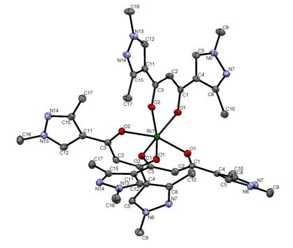
**Fig. 2** Molecular structure of **1** from the structure refinement of solvate **2**. The thermal ellipsoids are shown at the 50% probability level. Atoms color: Sc (green), N (blue), O (red), C (grey). The hydrogen atoms have been omitted for clarity.
