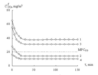
**Fig. 1** Time dependence of the final concentration of CO,  $C_{CO}^{f}$ , during the oxidation of carbon monoxide with oxygen over Pd(II)-Cu(II) catalysts based on natural (curve 1) and pre-modified bentonite (curves 2-4): 1 - N-Bent, 2 - 300-Bent,  $3 - H_2O$ -Bent, 4 - H-Bent-1.
