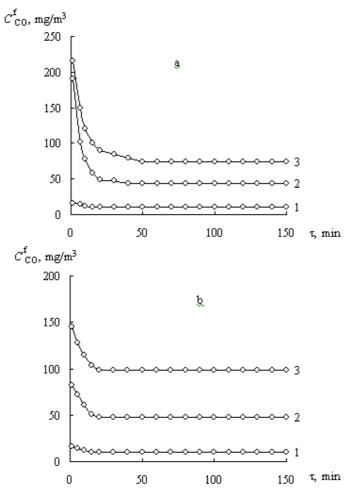
**Fig. 2** Time dependence of the final CO concentration in a  $K_2PdCl_4$ -Cu(NO<sub>3</sub>)<sub>2</sub>-KBr/H-Bent-1 sample in the process of oxidation of carbon monoxide with oxygen under different conditions of desorption of palladium(II) (a) and copper(II) (b): 1 – reference sample; 2 – desorption with water at 293 K; 3 – desorption with nitric acid at 373 K for 30 min.
