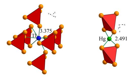
Fig. 5 Coordination surrounding of the Tl and Hg atoms by S atoms and by  $SnS_4^{4-}$  tetrahedra in the structure of  $Tl_2HgSnS_4$ .
