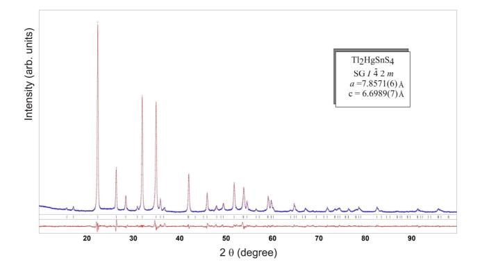
Fig. 2 Experimental (blue) and theoretical (red, top) diffraction patterns for  $Tl_2HgSnS_4$  and their difference (red, bottom).
