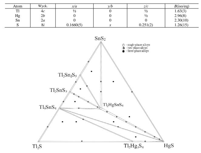
Table 3 Atomic coordinates and isotropic displacement parameters for Tl<sub>2</sub>HgSnS<sub>4</sub>.
