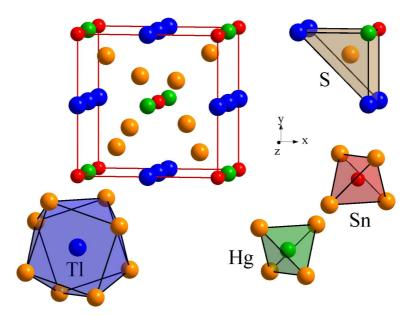
Fig. 3 Projection of the unit cell of  $Tl_2HgSnS_4$  onto the xy plane and the coordination polyhedra of the atoms.
