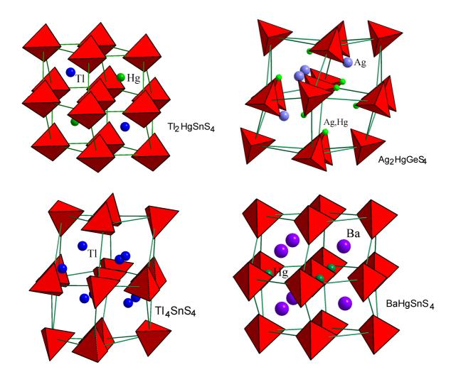
**Fig. 4** First (metal atoms) and second (other complex anions) coordination surroundings of the  $SnS_4^{4-}$  (GeS<sub>4</sub><sup>4-</sup>) anions in the structures of  $Tl_2HgSnS_4$ ,  $Ag_2HgGeS_4$ ,  $Tl_4SnS_4$ , and  $BaHgSnS_4$ .
