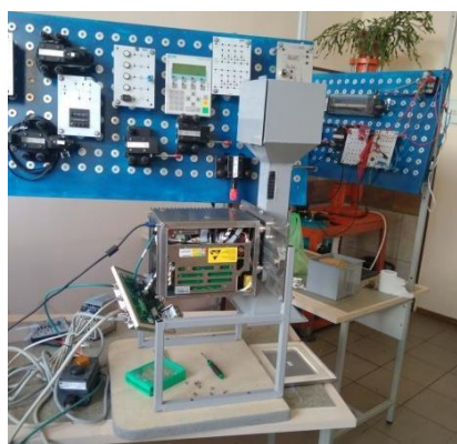
Fig. 6. The process of assembling a laboratory stand for the experiment: a) assembly stage; b) finished stand during research
