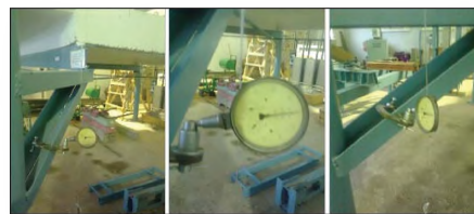
Fig. 2. Testing method for the thread of a composite material
