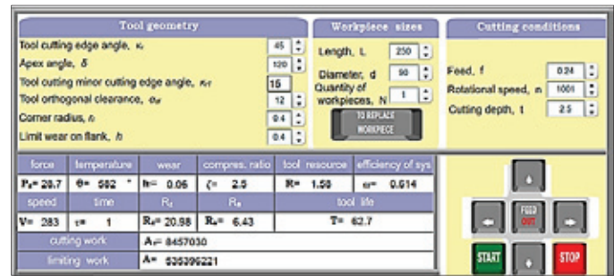
Fig. 3. Calculation of the turning process characteristics
