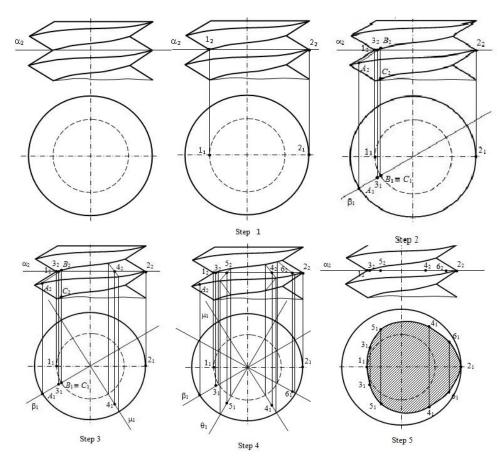
Fig. 2. Solution of a problem 81 of Chapter 8 «Cylindrical and conical helical lines and screws» [authoring]
