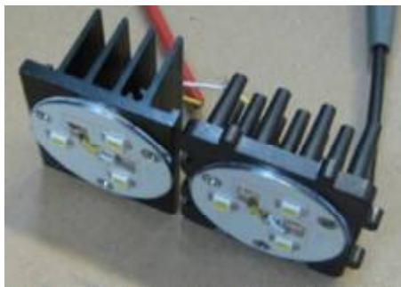
Fig. 1. Experimental samples with heat sinks made of aluminum (left) and composite (right).
