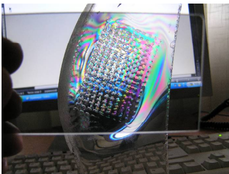
Fig. 4. Internal strains in organic glass after hot deformation.
