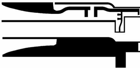
Fig. 3.2. Microwave mixer board.
