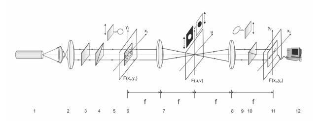
**Fig. 1.** Optical scheme of Fourier polarimeter: 1 – He-Ne laser; 2 – collimator; 3 – stationary quarter-wave plate; 5, 9 – mechanically movable quarter-wave plates; 4, 10 – polarizer and analyzer, respectively; 6 – object of study; 7, 8 – polarization microobjectives; 11 – CCD camera; 12 – personal computer.  $F(x_1, y_1)$  – object plane,  $F(x_2, y_2)$  – image plane, F(u, v) – Fourier plane with the diaphragms.
