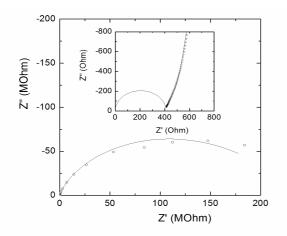
**Fig. 3.** Nyquist plot for  $Ag_7GeS_5I$ -based composite with the fitting result. A high-frequency magnified part of the plot is shown in the inset.
