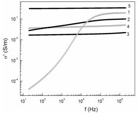
**Fig. 1.** Frequency dependences of the real part of electrical conductivity for composites based on  $(Ag_{1-x}Cu_x)_7GeS_5I$  mixed crystals:  $Ag_7GeS_5I$  (1),  $(Ag_{0.75}Cu_{0.25})_7GeS_5I$  (2),  $(Ag_{0.5}Cu_{0.5})_7GeS_5I$  (3),  $(Ag_{0.25}Cu_{0.75})_7GeS_5I$  (4) and  $Cu_7GeS_5I$  (5).
