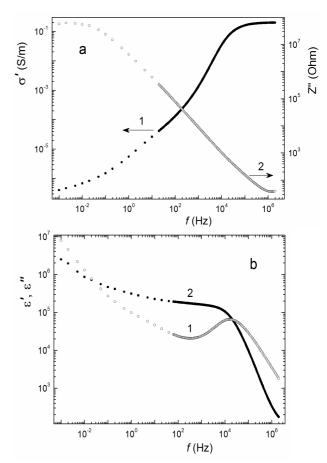
Fig. 2. Frequency dependences of the real part of electrical conductivity (1a), imaginary part of impedance (2a), real (1b) and imaginary (2b) parts of dielectric permittivity for  $Ag_7GeS_5I$ -based composite.
