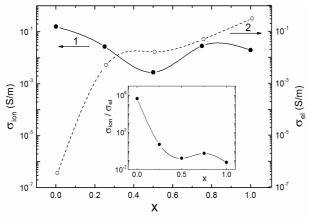
**Fig. 5.** Compositional dependences of ionic (1) and electronic (2) contributions to electrical conductivity for polymer composites based on  $(Ag_{1-x}Cu_x)_7GeS_5I$  mixed crystals. The inset shows the compositional dependence of ionic to electronic conductivity ratio for polymer composites based on  $(Ag_{1-x}Cu_x)_7GeS_5I$  mixed crystals.
