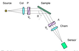
**Fig. 2.** Scheme of the experimental setup: collimator lens – Col, polarizer – P, analyzer – A, chamber lens – Cham.
