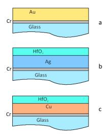
**Fig. 1.** Hybrid multilayer structure of the investigated samples based on Au (a), Ag (b) and Cu (c) thin films.
