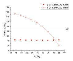
**Fig. 3.** Angular dependences of parameters  $\psi$  and  $\Delta$  for the Au (reference) sample.
