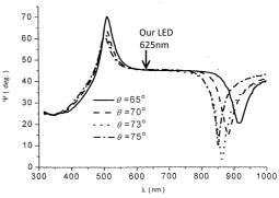
Fig. 7. Spectral dependences of ellipsometric parameter  $\psi$  of the heterostructure Cr (3 nm), Au (30 nm), HfO<sub>2</sub> (45 nm) for different angles of light incidence.
