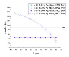
Fig. 4. Angular dependences of parameters  $\psi$  and  $\Delta$  for Ag-based samples.
