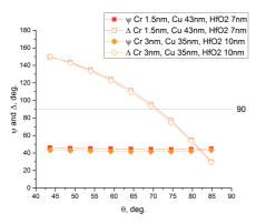
Fig. 5. Angular dependences of parameters  $\psi$  and  $\Delta$  for Cu-based samples.
