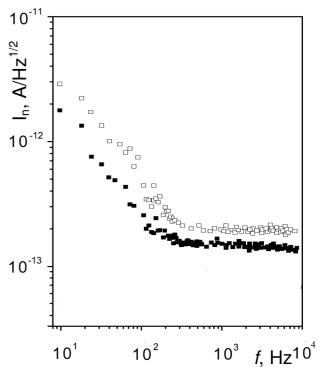
**Fig. 4.** Noise spectra measured in TR3 junction measured at the reverse bias -10 mV, T = 77 K.
