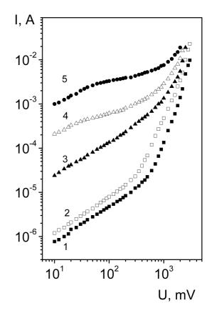
**Fig. 1.** Current-voltage characteristics in forward biased (close dots) and reverse biased (open dots) TR1 and TR3 junctions at 77 K.
