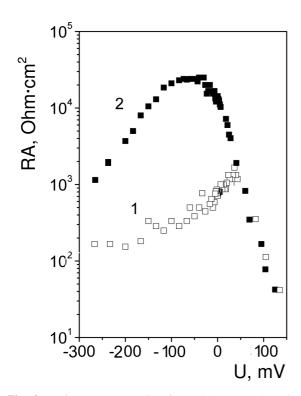
**Fig. 3.** Resistance-area product in TR1 (open dots) and TR3 (close dots) junctions at 77 K.
