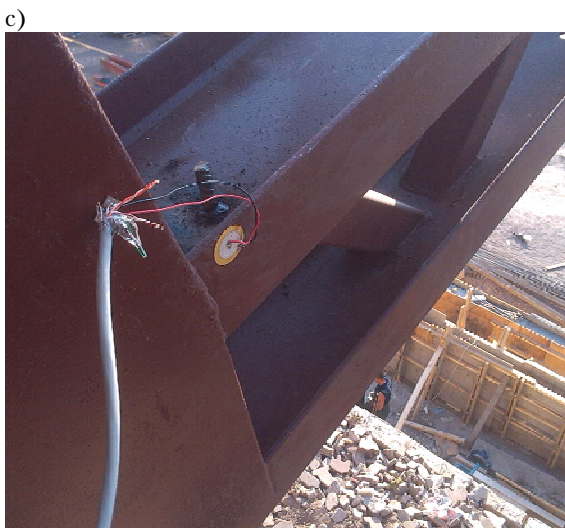
Figure 4. Registration of trusses vibration: a, b) placement of vibration machine on the trusses; c) installation of piezoelectric transducers; d) registration of vibrations.
