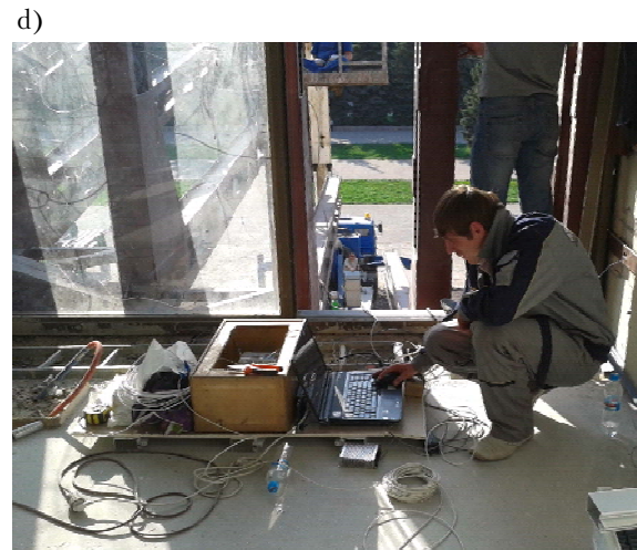
Figure 4. Registration of trusses vibration: a, b) placement of vibration machine on the trusses; c) installation of piezoelectric transducers; d) registration of vibrations.
