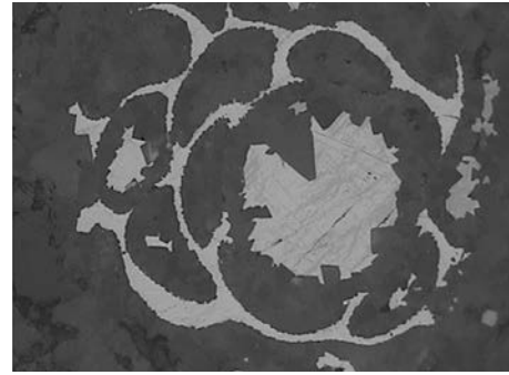
Fig. 9. Low temperature intergrowth of sphalerite (grey) with galena (white) and chalcopyrite in dolomite sparite, Rudna Mine. Reflected light, \times 600 .
