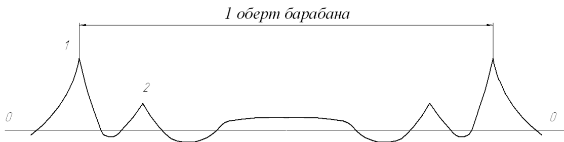
Fig. 7. Working waveform of bending stresses in the drum
